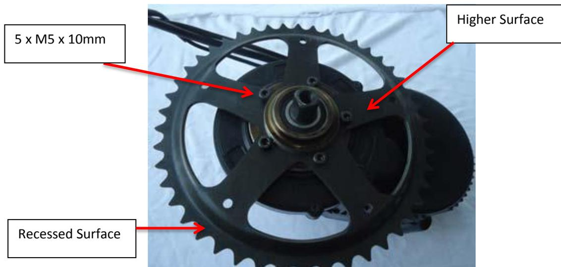
3. Carefully feed the drive unit axle through the bottom bracket. If you encounter resistance your BB shell may need to have burrs / weld overflow smoothed with a rounded file.
