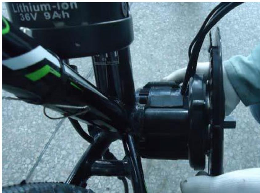
Make sure the thread of the axle tube extends beyond the bottom bracket more than 10mm. Please note that for 73mm bottom brackets this may be less.
